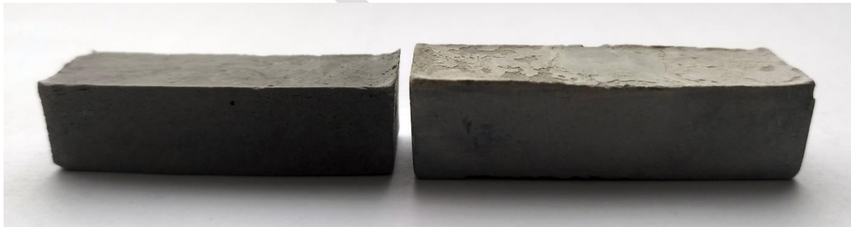
Fig. 5. Visual appearance of GS 20 F 0.5 (left) and PS 20 F 0.5 (right) composites
