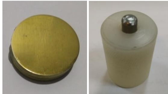
Fig. 7. Type I projectile with pin-shaped steel bullet (right) and TiN coated steel specimen (left)
