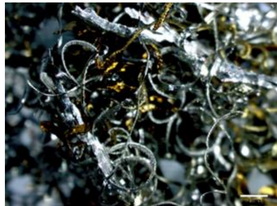
Fig. 1. AA 7075 swarf produced from the machining process
