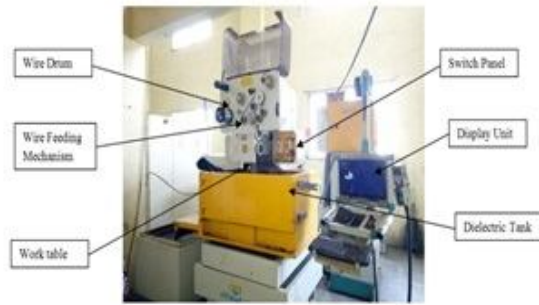
Fig. 2. Wire-Cut EDM set up photograph
