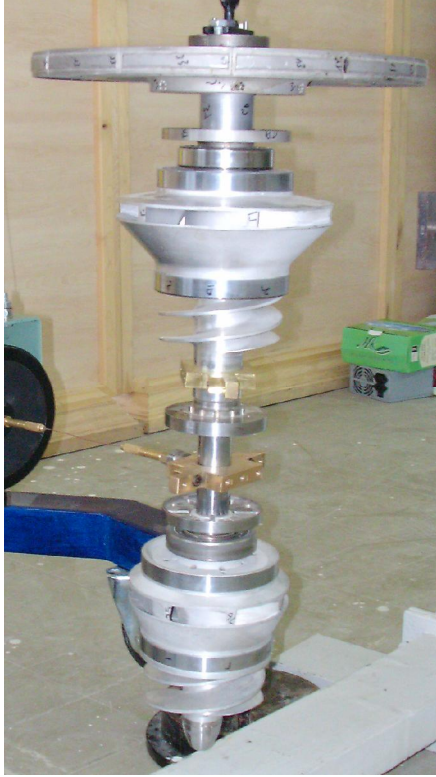
Fig. 1. The Shaft and corresponding components of turbo-pump
