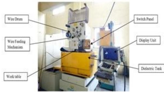
Fig. 2. Wire-Cut EDM set up photograph
