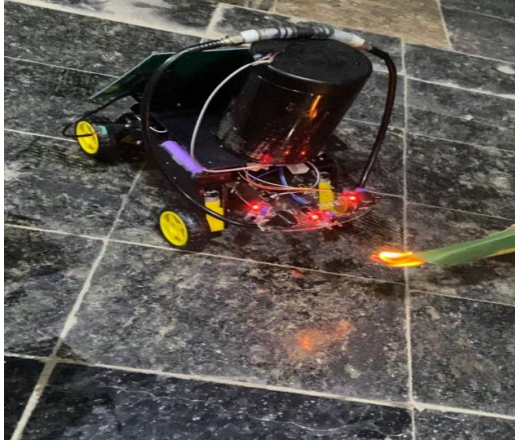
Fig. 16 Fire Fighting robot implementation.
