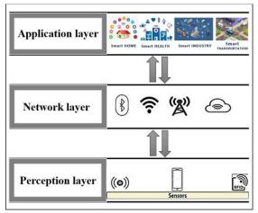
Fig. 1 The three-layered architecture of IoT.
