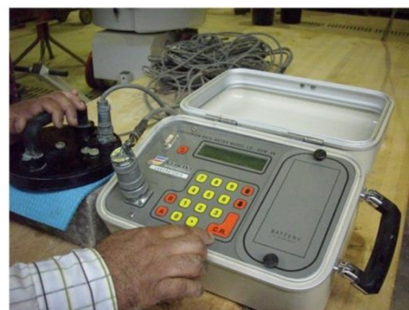
Figure 4 GECOR-8 (Corrosion Measurement device)
