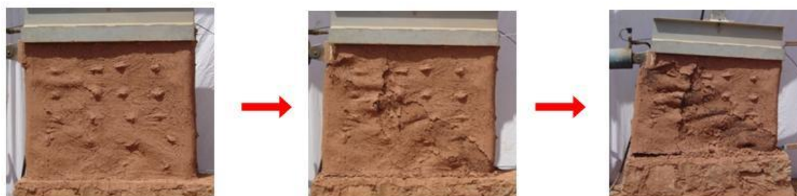
Fig. 15 Damage mechanism of RMW1 wall
