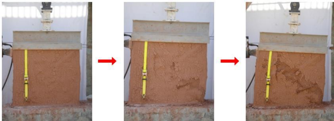
Fig. 18 Damage mechanism of RMW2 wall
