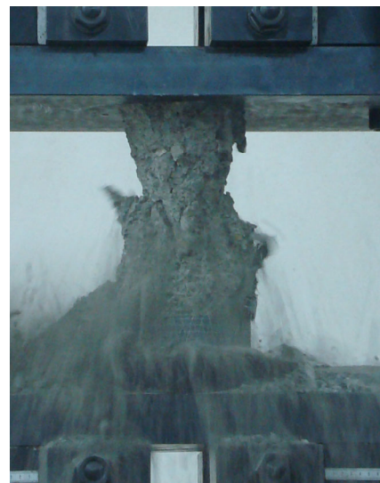
Fig. 7. Abrupt failure mode of FRP strengthened specimen
