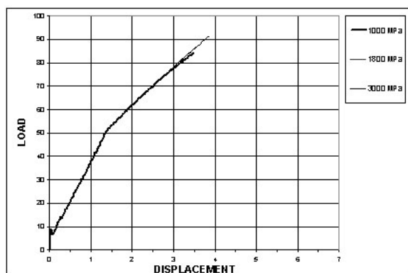
Fig. 12. Load-deflection curves for beams with different CFRP ultimate strength.
