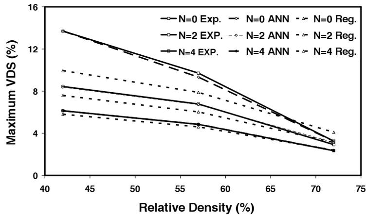
Fig. 9. comparison of ANNs and regression model predicted with experimental data of VDS versus soil relative density.
