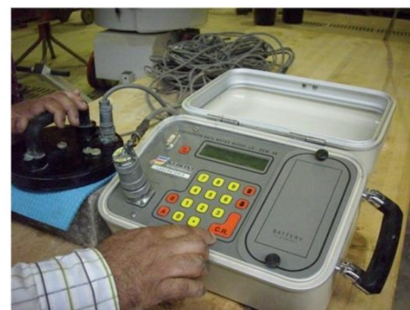
Figure 4 GECOR-8 (Corrosion Measurement device)
