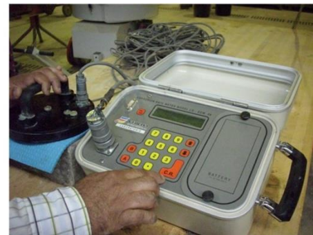
Figure 4 GECOR-8 (Corrosion Measurement device)
