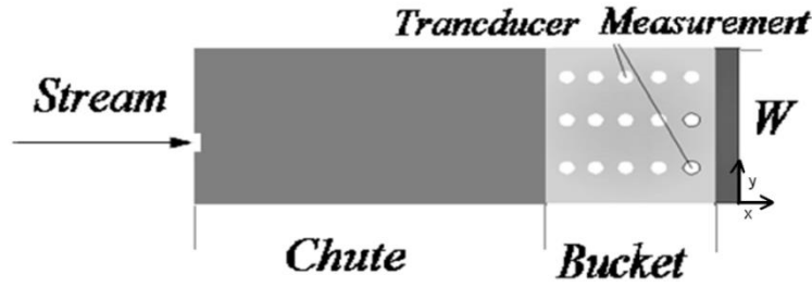
Fig. 3 Plan view of pressure transducer locations over flip bucket bottoms
