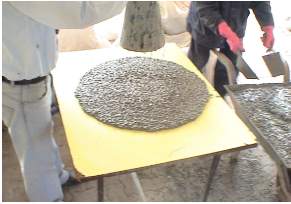
Fig. 2. Slump flow test of SCLWC
