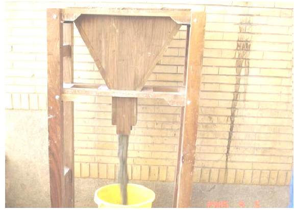
Fig. 4. V-funnel test of SCLWC
