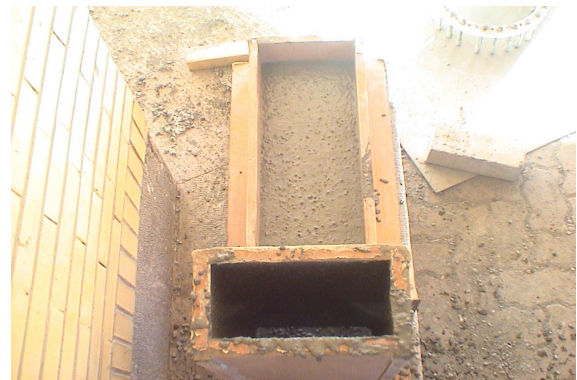
Fig. 5. L-box test of SCLWC
