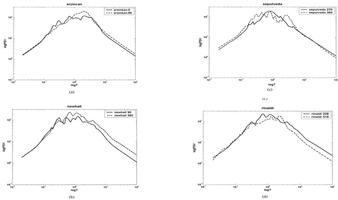
**Fig.1** comparison pseudo velocity spectra of fault-normal and fault-parallel components of near-fault motion recorded at (a) Erzincan station (b) Newhall station (c) Sepulveda station (d) Rinaldi station
