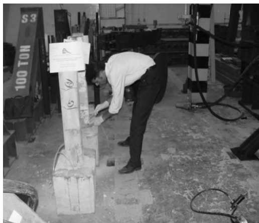
Fig.8 Cleanig surface of the damaged columns
