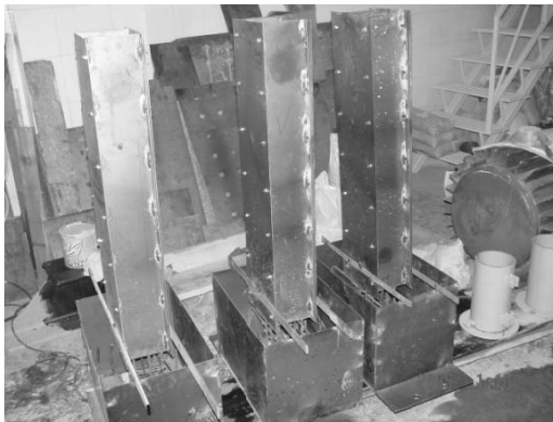
Fig.3 Specimens reinforcing cage in their formworks
