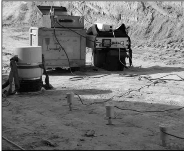
Fig. 3. Surface wave attenuation measurements at the site
