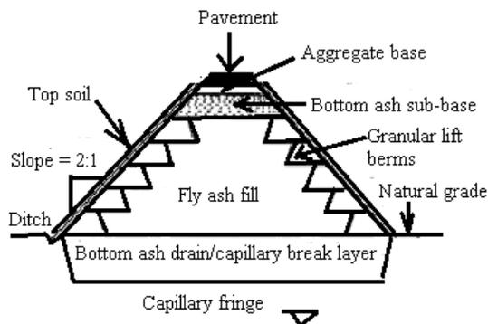
Fig. 2 (a) Fly ash in embankment
