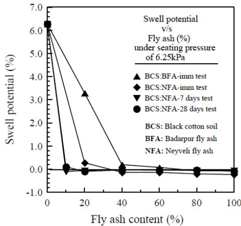
Fig. 7(a) Effect of fly ashes on swelling characteristics of BC soil
