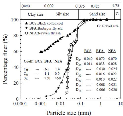
**Fig. 3** Particle size distribution curves for BC soil and Fly ashes
