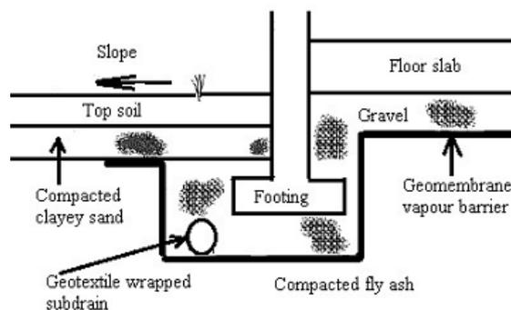
Fig.2 (b) Building foundation using fly ash
