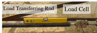
f. Instrumentation, Load Cell
