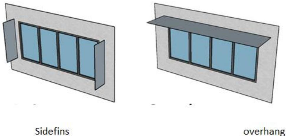
**Fig 6.** The Shading Device Types of Side Fins and Overhangs
