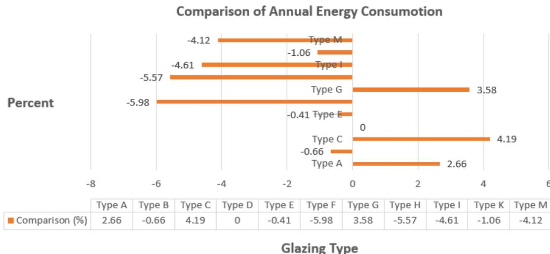
Fig 4. Comparison of Annual Energy Consumption with Variant Glazing Types
