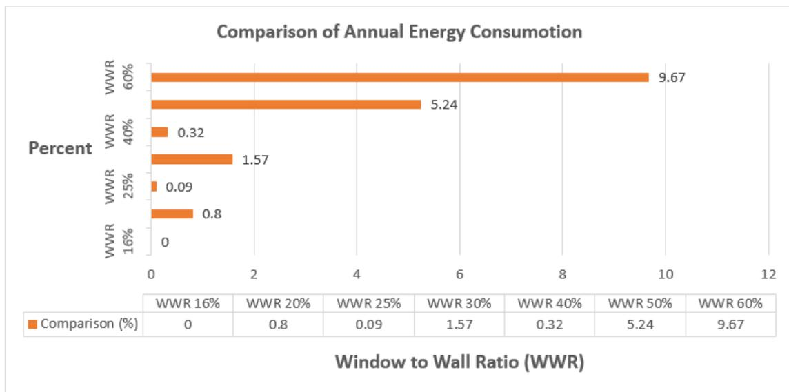
**Fig 5.** Comparison of Annual Energy Consumption with variant Window to Wall Ratio (WWR)
