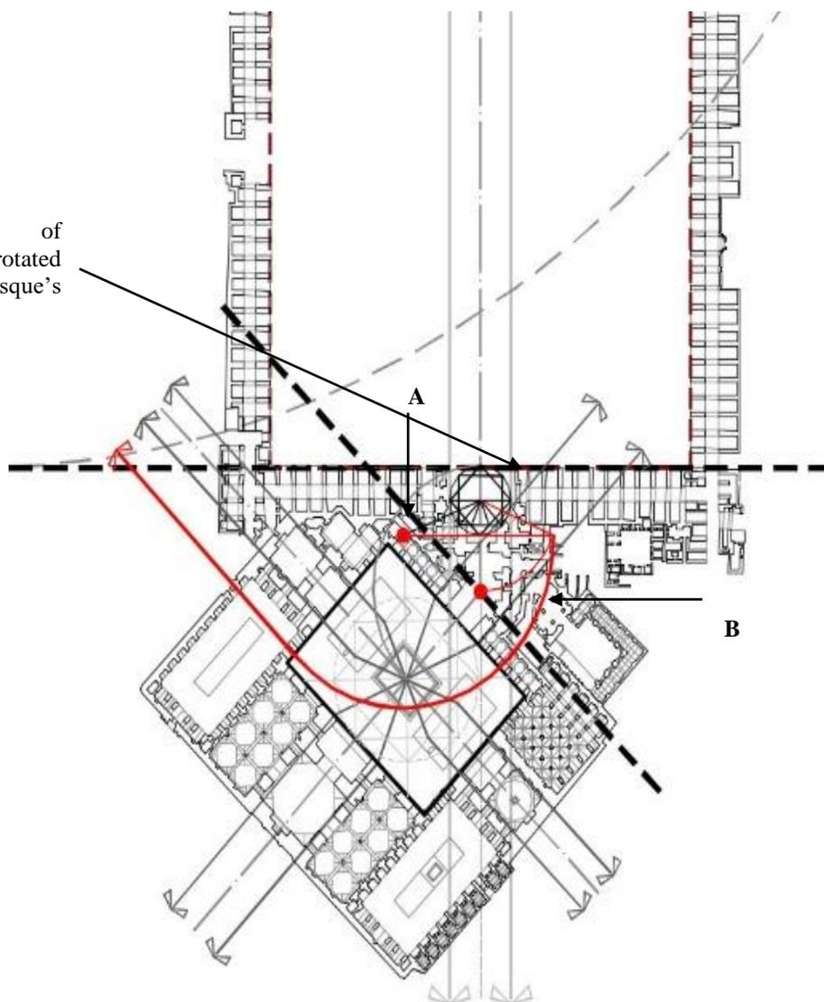
**Fig 7.** Determination of the width of the courtyard of the *Abbasi Jamee mosque* based on the Relative square Measuring System (congruent rotated squares) on the entrance of the building (writers) g
