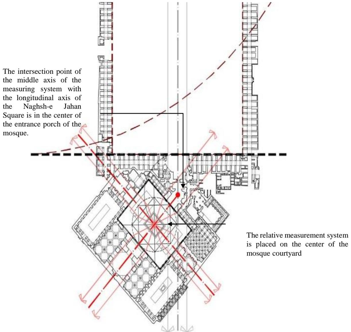
**Fig 5.** Positioning the Relative square Measuring System on the geometric center of the of *Abbasi Jamee mosque* (writers)
