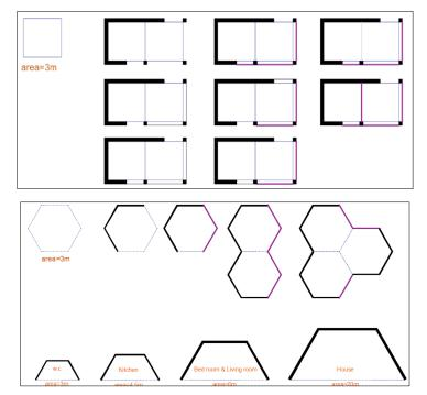
Fig 2. Specification of Square and Hexagonal Modules for the Design of Plan (Source: Authors)
