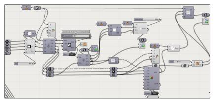
Fig 1. An Algorithm for Drawing a Schematic Plan of Spatial Layout via Space Syntax Plugin and Grasshopper
