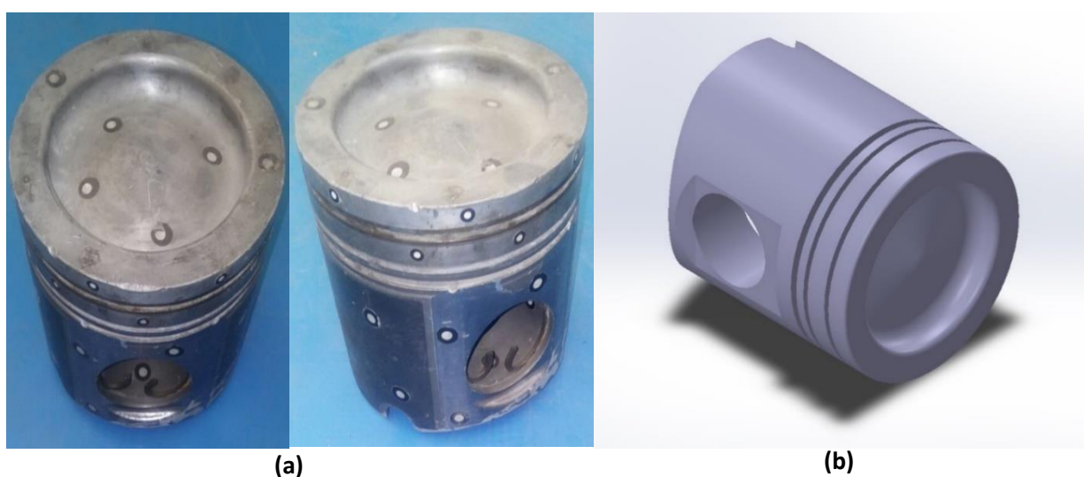
Figure 1: OM457's piston head a: real one – b: .stl file of OM457's piston head used for CFD analyses
