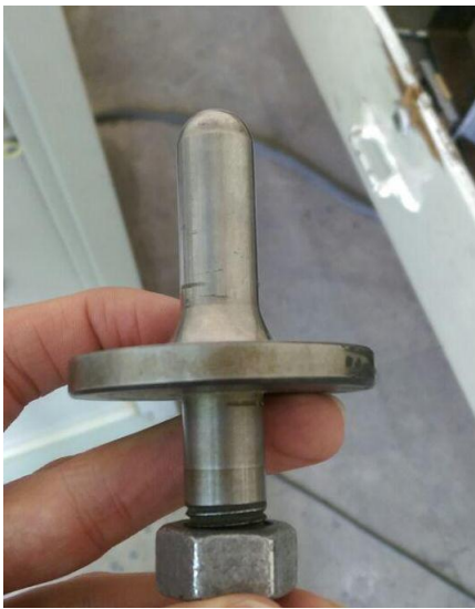
Fig2.Steel imp actor used in drop ball tests
