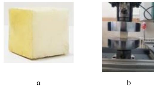
Figure 3: (a) a polyurethane foam sample, (b) compression testing machine.
