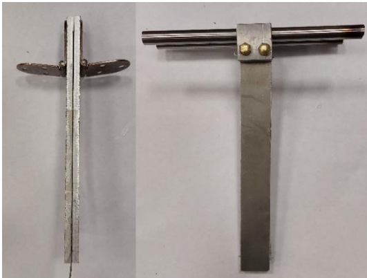
Figure 5: Specimens for static and impact loading
