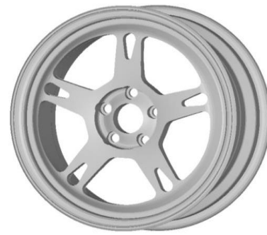
Figure 20: The optimized design after topology optimization
