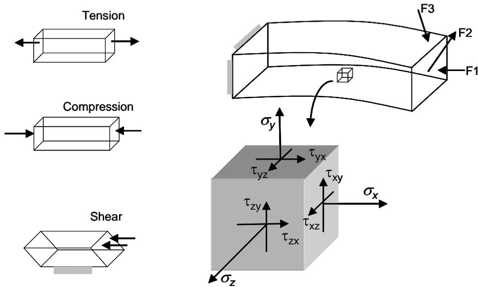
Figure 3. Tensile, compressive and shear stresses; stresses in an infinitesimal element of a beam
