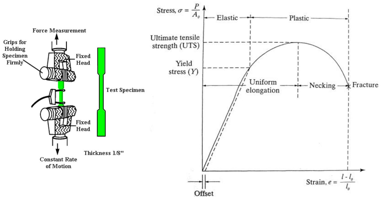
Figure 5. (a) Schematic of a tensile test
