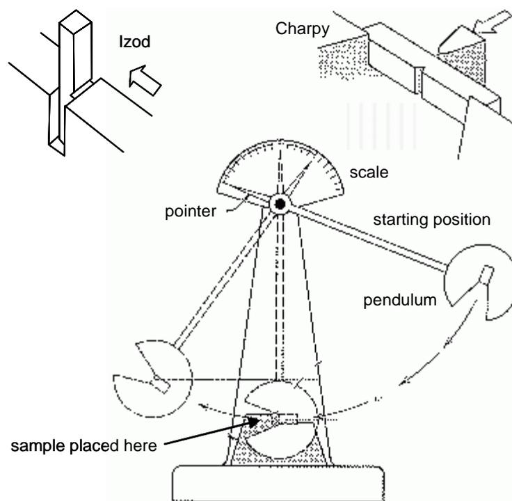
Figure 11. The setup for Charpy and Izod tests for Impact strength
