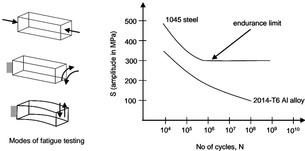
Figure 10. Modes of fatigue testing, and typical SN curve for compressive loading case
