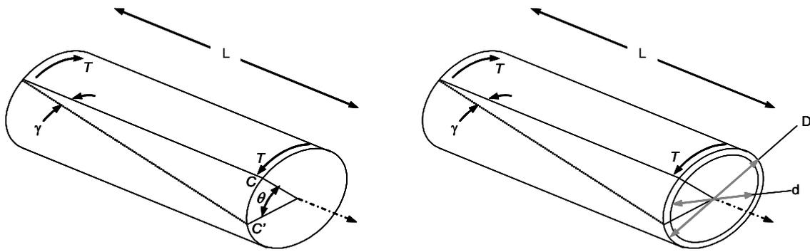
Figure 9 (a). Solid cylinder under torsion (b) Thin walled cylinder under torsion
