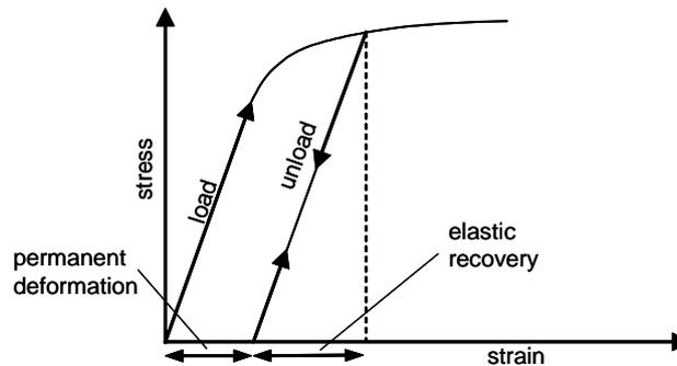
Figure 6. Elastic recovery after plastic deformation
