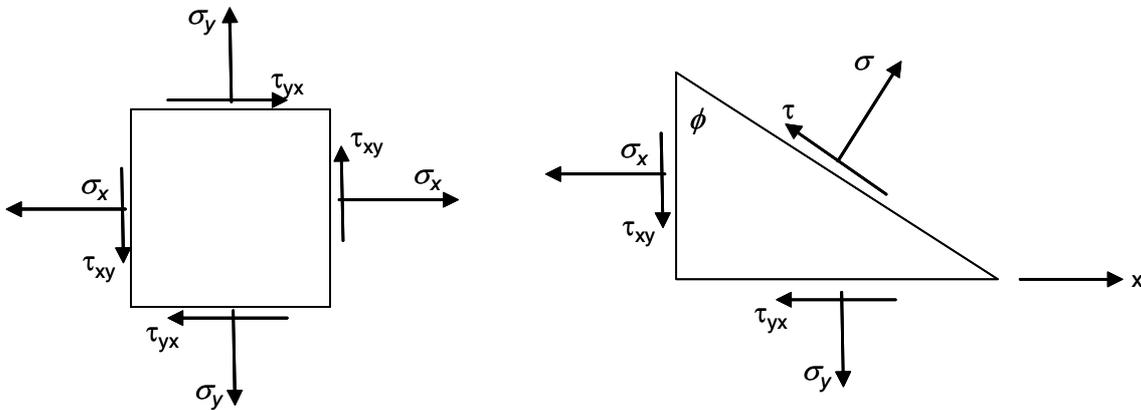
Figure 4. Computing the principal stresses (2D case)
