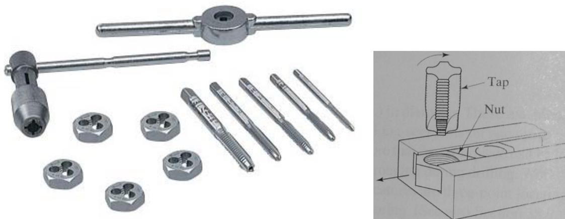
Figure 8. Thread-cutting. A drilled hole can be given internal threads by using a tapping tool; external threads on a cylindrical shape are made using a tapping die. The left image shows manual tool set for making external and internal threads. The right image shows a schematic for automatic tapping of threads in nuts.
