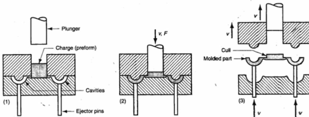
FIGURE 8. Schematic of Transfer Molding
