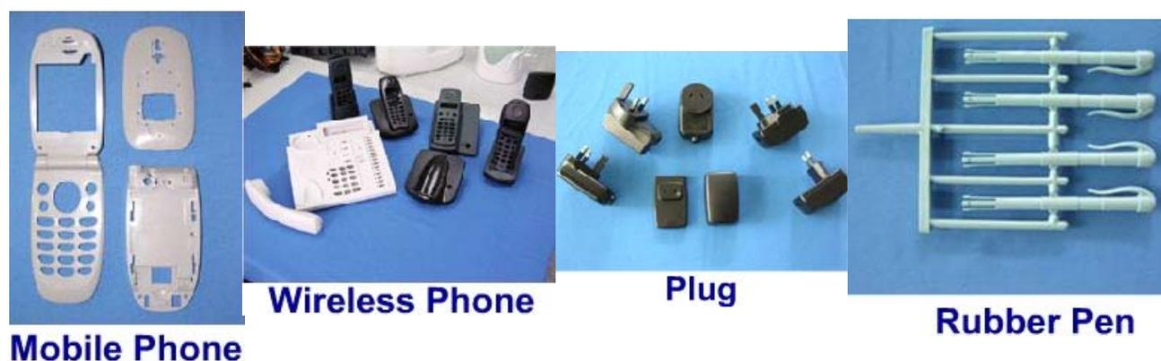
Figure 11. Examples of Injection Molding Parts [source: [www.ylmf.com.hk](http://www.ylmf.com.hk)]
