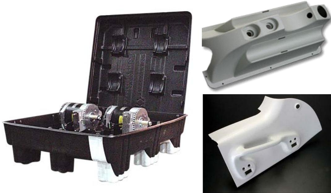
Figure 5. Thermoformed parts
