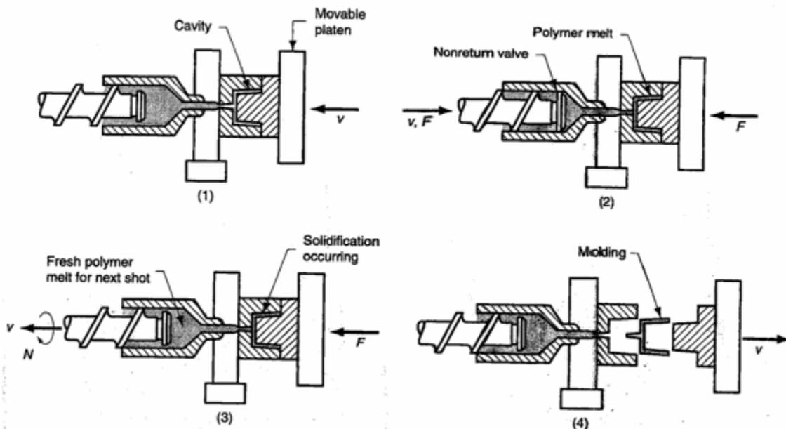
Figure 10. Cycle of operation for injection molding [source: [www.offshoresolutions.com](http://www.offshoresolutions.com)]
