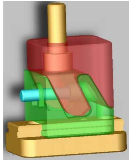
Figure 14 (a). A mold with four side action cams (b) The operation of side action cams
