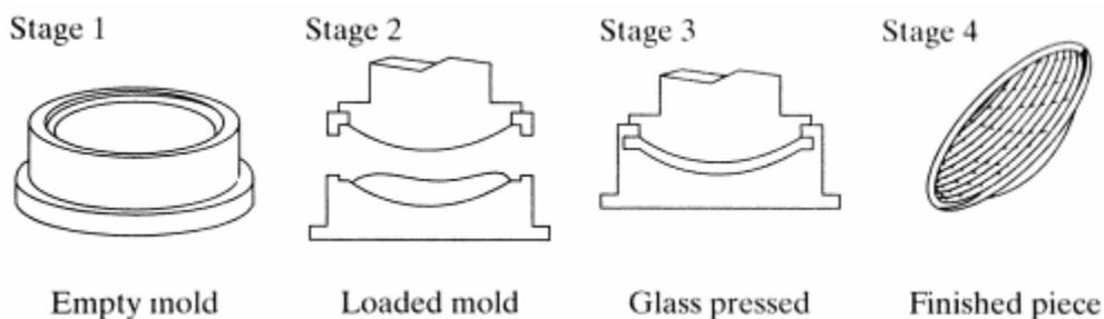
Figure 4. Molding of lenses [source: Kalpakjian & Schmid]
