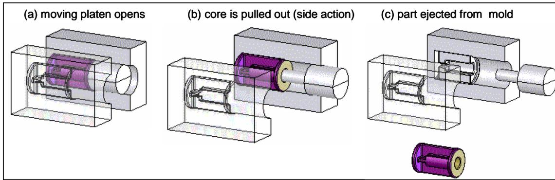
Figure 13. Injection molding a part with side action using core
