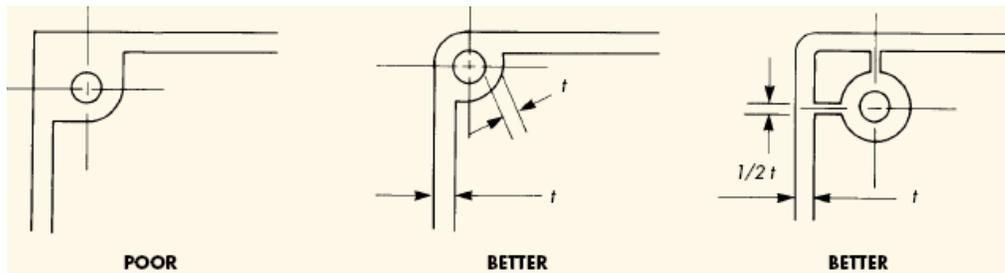
Figure 23. Example of improving design for injection molded parts
