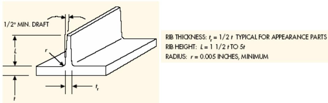
Figure 21. Guidelines for rib dimensions
