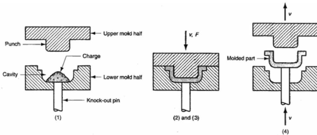
Figure 7. Schematic of Compression Molding
