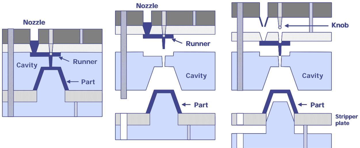
Figure 17. The mold in operation
