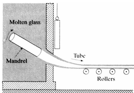
Figure 3. Drawing of glass tubes [source: Kalpakjian & Schmid]
