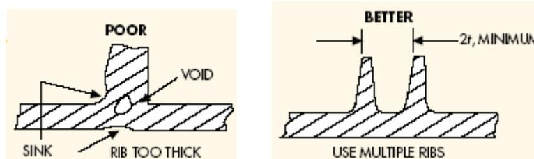
Figure 22. Molding problems (sink holes and voids) occur if the part has thick sections
