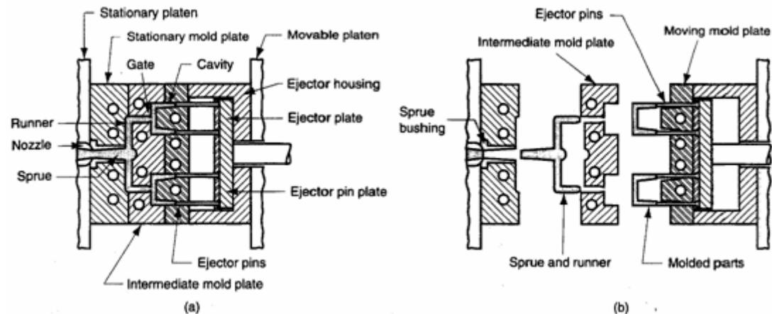
Figure 12(b). A three-plate mold
