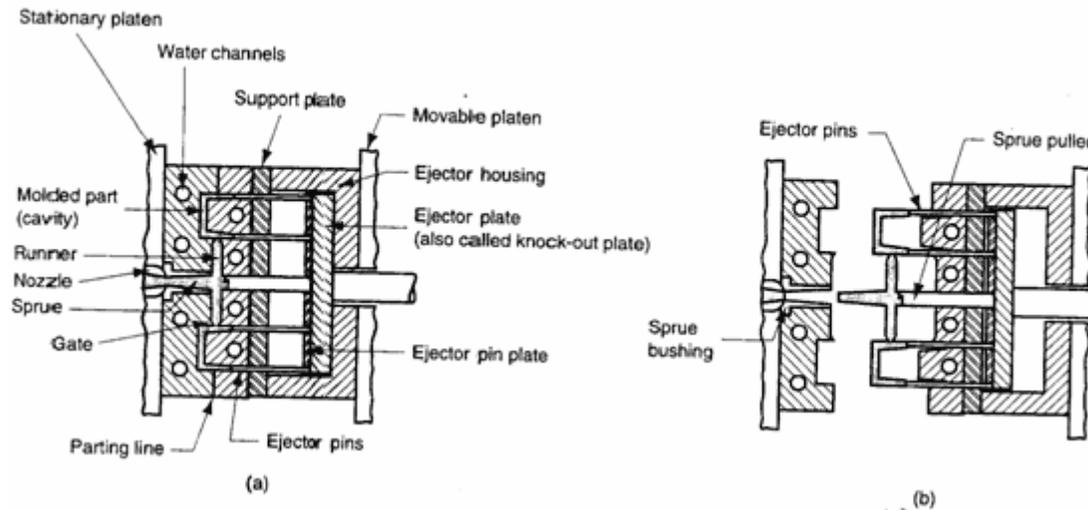
Figure 12(a). A two-plate mold
