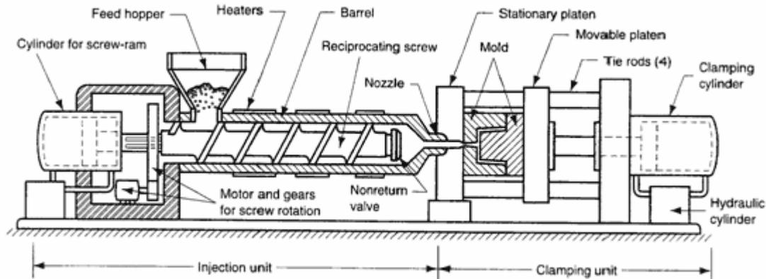
Figure 9. A simple reciprocating screw injection molding machine [source: [www.offshoresolutions.com](http://www.offshoresolutions.com)]
