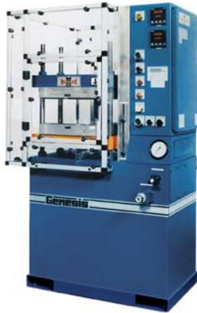
Figure 6. A compression molding machine
