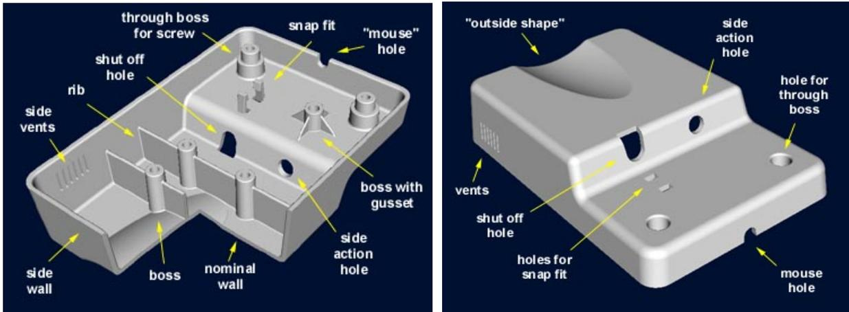
Figure 18. Examples of different shape features in typical injection molded parts [source: www.idsa-mp.org]
