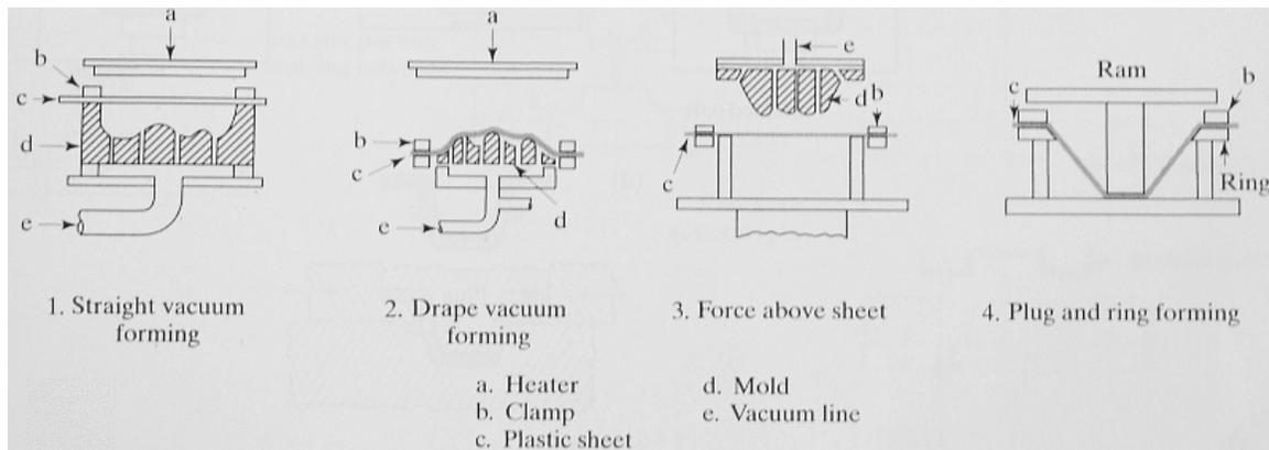
Figure 3. Schematic of thermoforming processes [source: Kalpakjian and Schmid]
