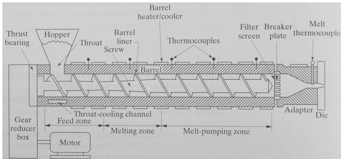
Figure 1. Extrusion machine schematic [source: Kalpakjian and Schmid]
