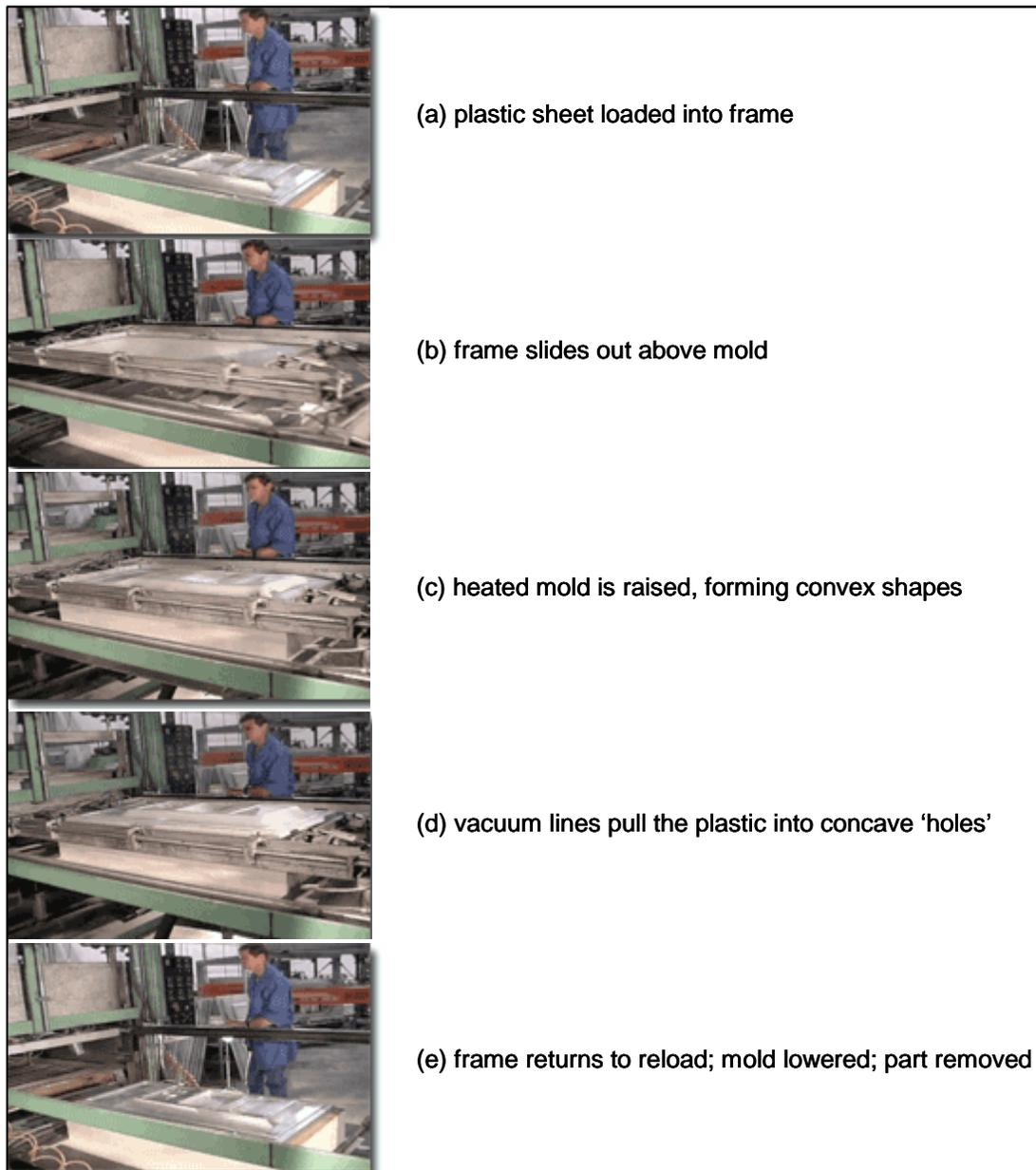
Figure 4. Stages in a vacuum thermoforming process [source: [www.ymlf.com.hk](http://www.ymlf.com.hk)]
