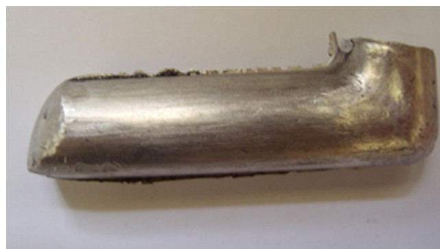
Fig. 2. The deformation shape of sample after 1 pass ECAPed.
