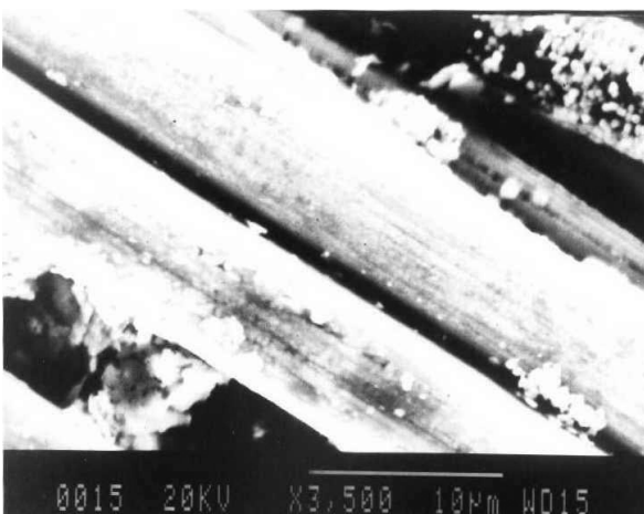
Fig. 9 The longitudinal SEM micrograph of carbon fibers coated with 1.1 μm thickness of nickel
