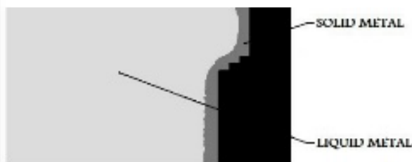
SECTION OF CASTING NEAR MOLD WALL SHORT TIME AFTER POURING
