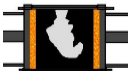
MOLD FOR SLUSH CASTING IMMEDIATELY AFTER POURING
