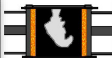
MOLD FOR SLUSH CASTING CROSS SECTIONAL VIEW OF INSIDE OF CASTING A CERTAIN AMOUNT OF TIME ( T_2 ) AFTER POURING ALSO NOTE ( T_2 > T_1 )
