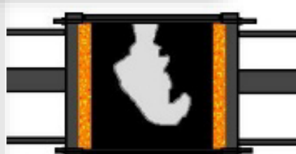
MOLD FOR SLUSH CASTING CROSS SECTIONAL VIEW OF INSIDE OF CASTING A CERTAIN AMOUNT OF TIME ( T_1 ) AFTER POURING
