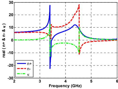
Fig. 2. The real parts of the RCP and LCP refractive indices and the chirality parameter of dendritic fractal CMM structure.
