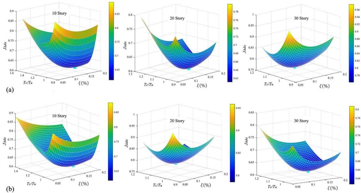
Figure 5. Variation of optimum parameters with respect to average displacement objective function a) N-Panel PMD model, (b) 1-Panel PMD model
