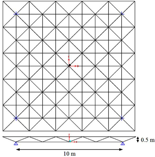
Figure 2. Configuration of the 200-bar double layer grid
