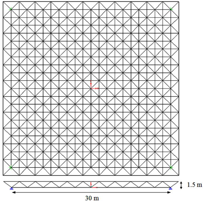
Figure 4. Configuration of the 968-bar double layer grid
