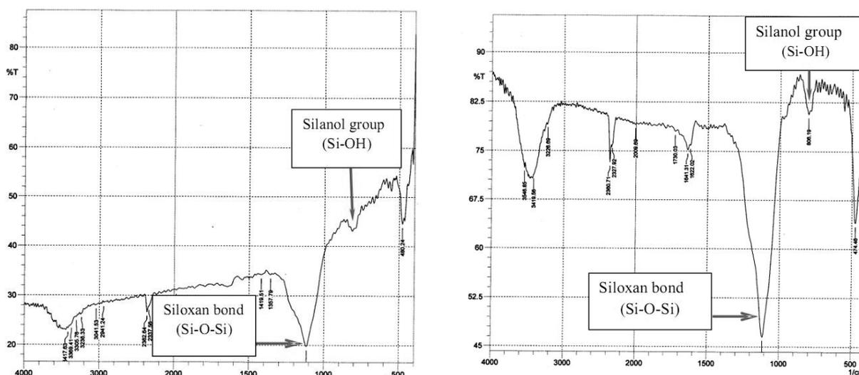
Fig. 8. a) Shallow valley in FTIR graph for Ce-CS sample shows the higher amount of siloxane bond (b) the deep valley for CS sample shows the lower content of siloxane bond.
