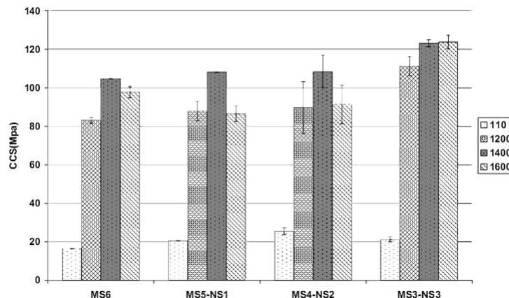
Fig. 2a. Cold Crushing Strength (CCS) for all specimens at different sintering temperatures
