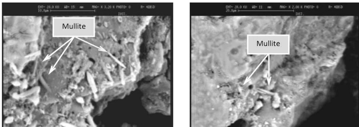
Fig. 5. a) Microstructure of the MS4-NS2 sample (b) the MS5-NS1 sample after sintering at 1400 °C showing well-growth mullite crystals
