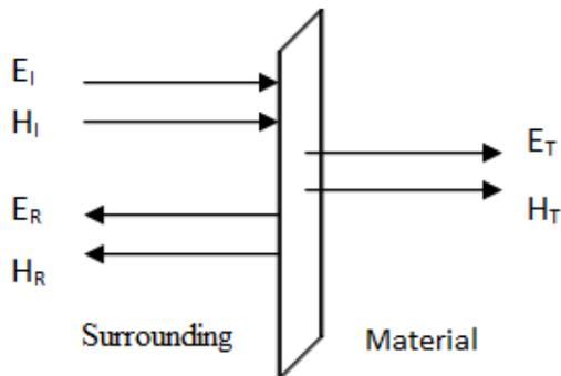
Fig. 2. Different waves at the material surface.
