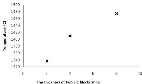
Fig. 17. Temperature at different SiC block sizes
