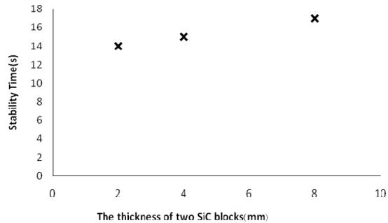
Fig. 16. Stability time at different SiC block sizes.
