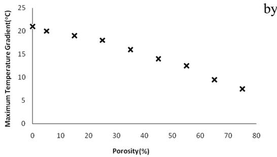
Fig. 12. Maximum temperature gradients at different porosity values.
