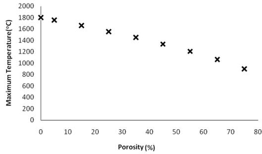
Fig. 11. Maximum temperatures at different porosity values.
