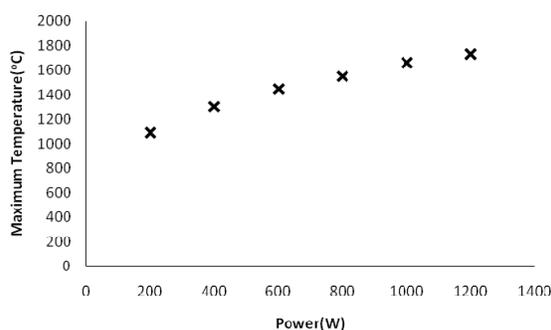
Fig. 8. Maximum temperatures at different input powers.
