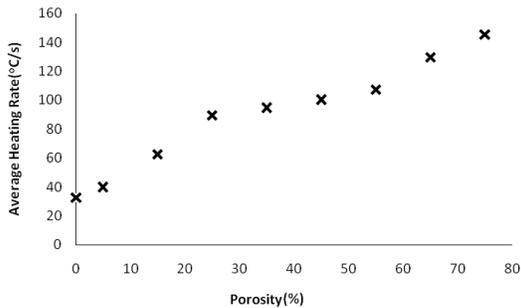
Fig. 13. Average heating rates at different porosity values.
