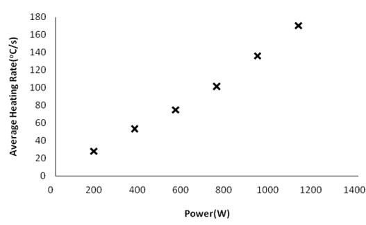
Fig. 10. Average heating rates at different input powers.
