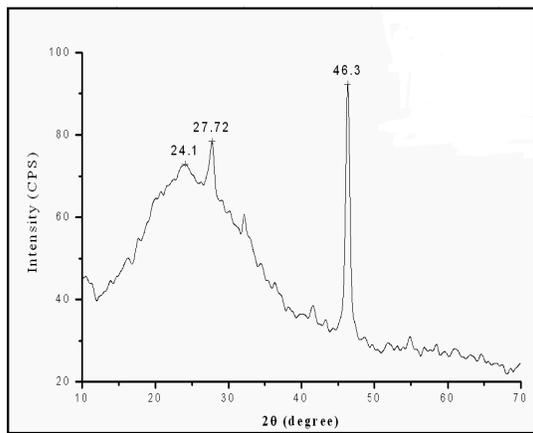
Fig. 2. XRD pattern of Cu<sub>2</sub>S thin films of 7000 Å thickness
