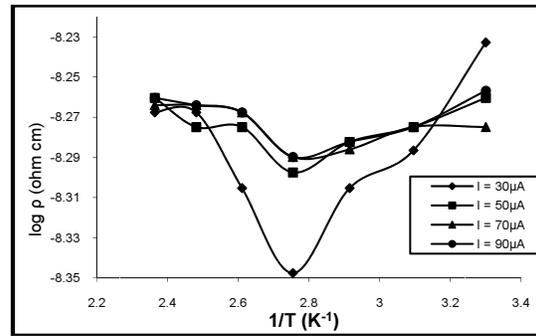
Fig. 3. Variation of resistivity with Inverse of temperature for Cu<sub>2</sub>S film of 1000 Å thickness
