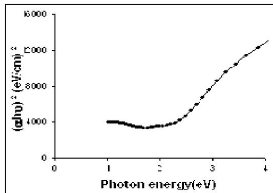
Fig. 7. Plot of  $(\alpha h \nu)^2$  versus  $h \nu$  for Cu<sub>2</sub>S thin film of 1000 $\text{\AA}$  thickness showing direct edge at 1.8 eV.
