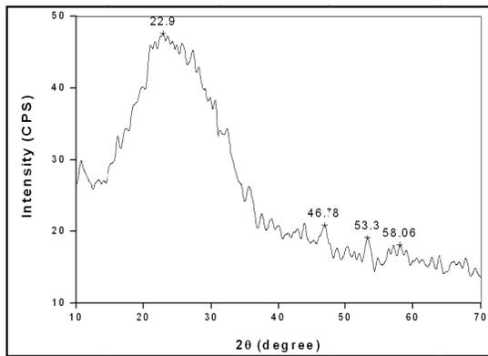
Fig. 1. XRD pattern of Cu<sub>2</sub>S thin films of 1000 Å thickness
