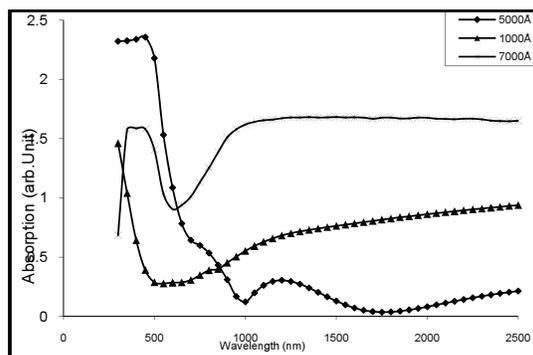
Fig. 6. Variation of absorbance spectra with wavelength for Cu<sub>2</sub>S films of different thicknesses
