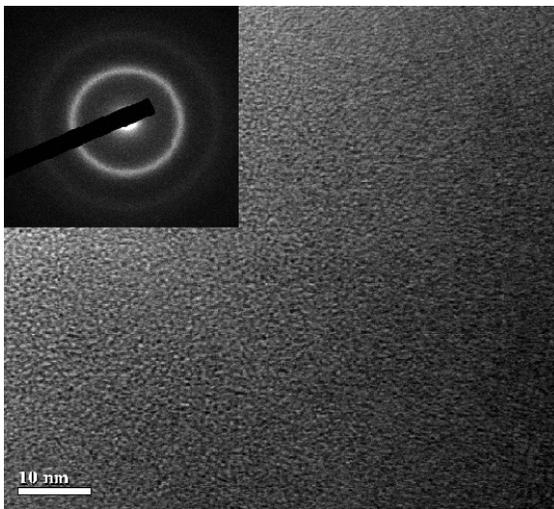
Fig. 6. Microstructure of the alloy in amorphous state.
