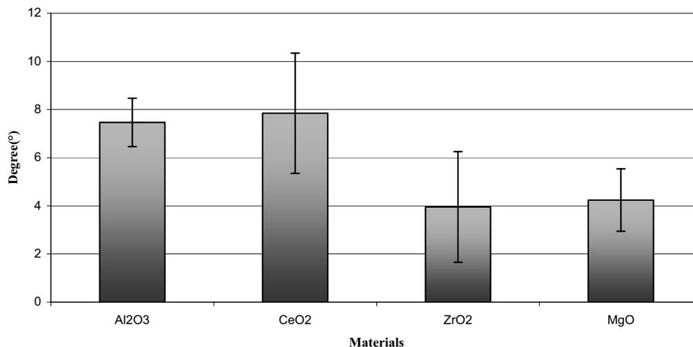
Fig. 9. Contact Angle of Na<sub>2</sub>CO<sub>3</sub> on dense candidate oxides.
