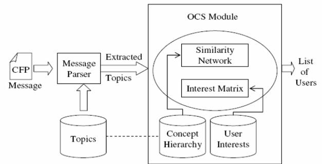
Fig. 4. System architecture [16]
