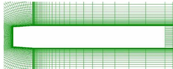
Fig. 3. Grid clustering near the solid wall boundaries
