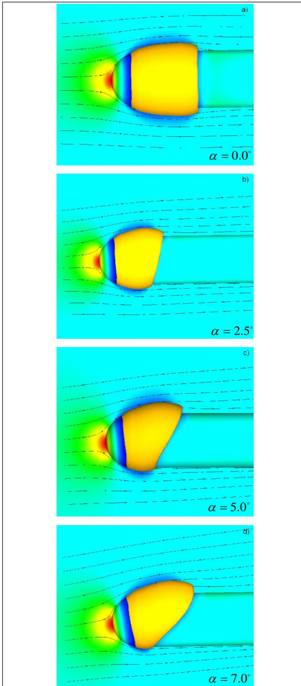
**Fig. 12. Predicted three-dimensional flow fields with natural cavitation about hemispherical fore-body at various angles of attack**
