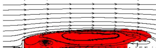
**Fig. 13. Supercavity shape behind a disk at  $\sigma = 0.15$**
