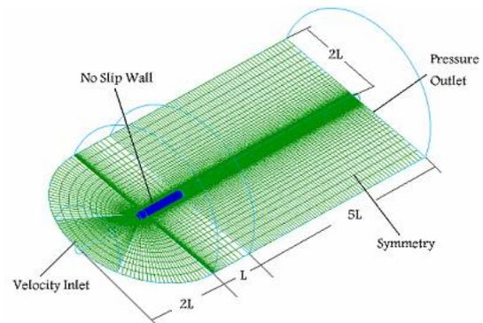
Fig. 2. Applied boundary condition for 3D computations
