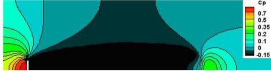
Fig. 15. Pressure coefficient for disk cavitator at  $\sigma = 0.15$
