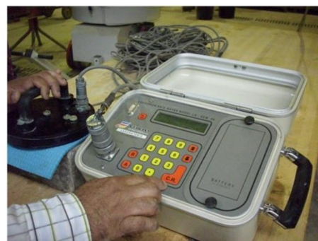
Figure 4 GECOR-8 (Corrosion Measurement device)
