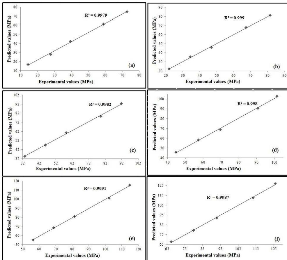
**Fig. 3** Predicted and experimental compressive strengths of CAPHSC mortar for Blaine finesses of (a) 205, (b) 250, (c) 303, (d) 351, (e) 400, and (f) 450 m<sup>2</sup>/kg
