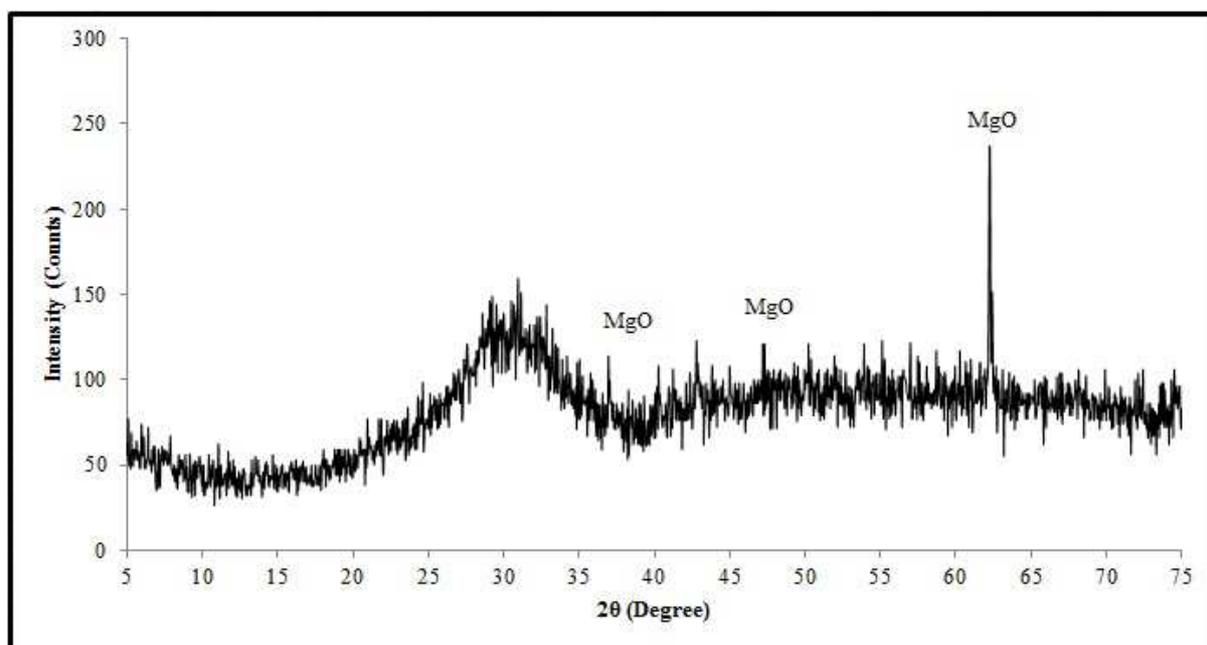
**Fig. 1** X-ray diffraction pattern of phosphorous slag
