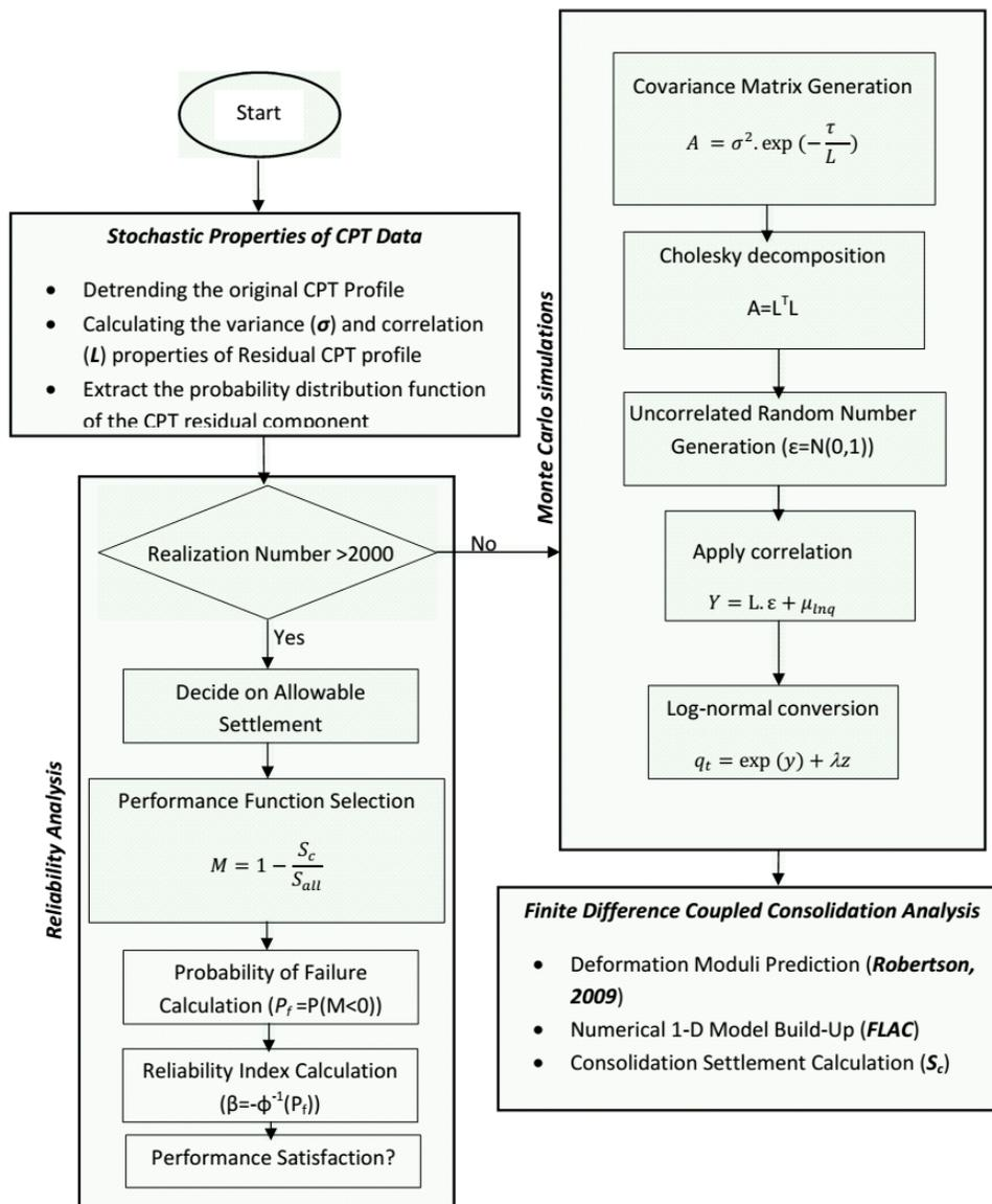
Fig. 7 Flowchart for calculation process of reliability analysis for consolidation settlement
