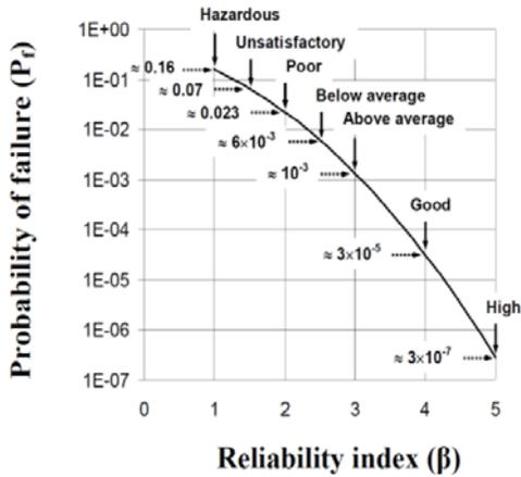
Fig. 5 Probability of failure versus reliability index according to USACE standard (Phoon, 2004)
