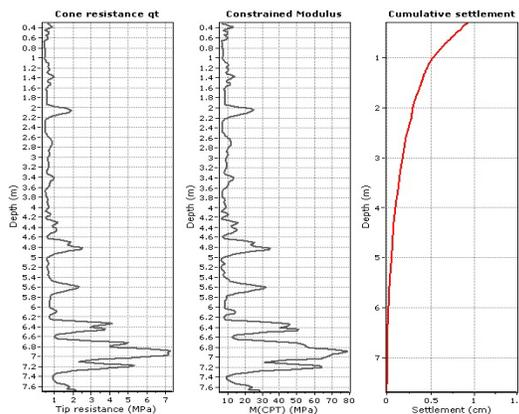
Fig. 8 Consolidation settlement prediction from deterministic analysis
