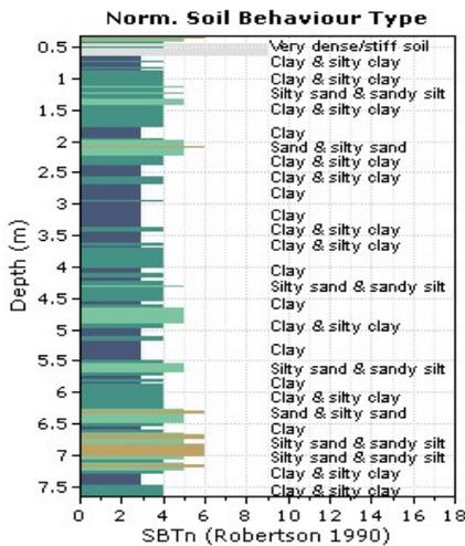
Fig. 1 Normalized soil behavior type based on CPT profile
