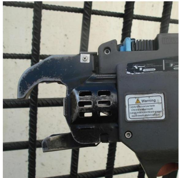
Fig. 4 Close-up of the adjustable pick
