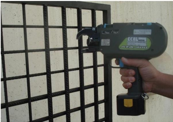
Fig. 6 Battery powered rebar tier
