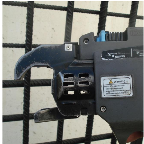
Fig. 4 Close-up of the adjustable pick
