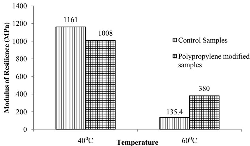
**Fig. 7** Resilient Modulus of control and modified samples
