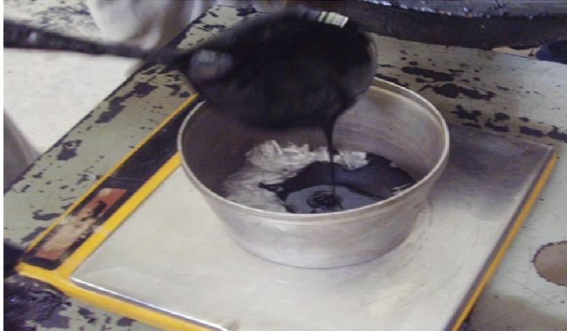
**Fig. 3** Mixing asphalt binder and fibres
