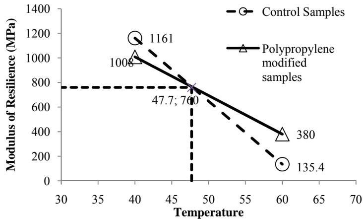
Fig. 8 Temperature and IDT strength correlation for control and modified samples
