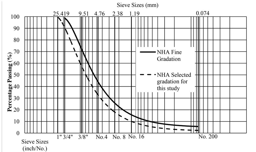
Fig. 1 Aggregate gradation curve
