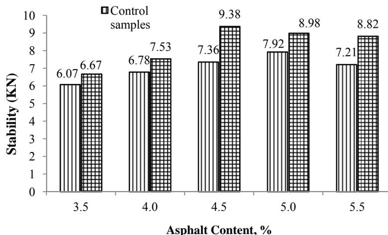
Fig. 4 Marshall Stability of control and modified samples
