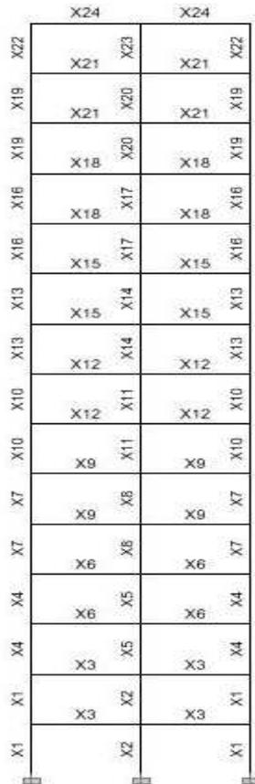
Fig. 8 Member grouping for the 15-Storey example
